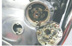
Remove the fixing bolt in the centre of the AAU. A threaded rod or bolt then goes into the AAU to assist removal. The AAU fits into a taper in the exhaust cam and may be difficult to remove.
