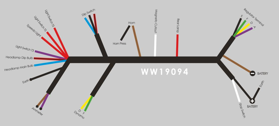
NB. for detailed information please refer to OEM wiring schematic
