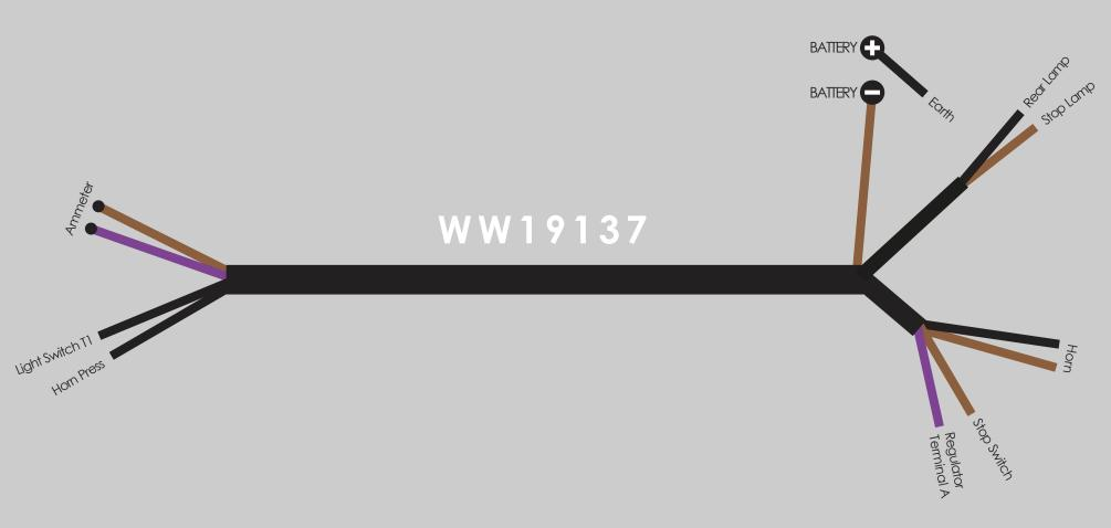
NB. for detailed information please refer to OEM wiring schematic
