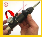
5. Fit the Allen screw (ideally apply Loctite CV), making sure that the screw properly locates in the slot. Remove the boot and check the distance between the end of the cast mounting bracket and the face of the pushrod nut. This dimension must be adjusted if necessary to 8.9 - 9.4mm (0.35" - 0.37").
