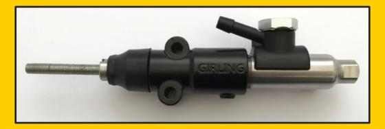
When the brake pedal is operated the piston moves along the bore to displace hydraulic fluid under pressure to operate the caliper pistons. On releasing the brakes, the return spring moves the piston back faster than the fluid can return and this causes the lip of the main rubber cup to relax. Fluid then passes over the cup from behind, through the holes drilled in the piston head for this purpose.
